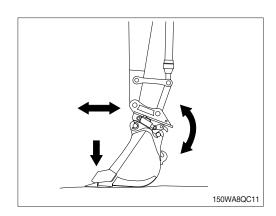
(14) Visually check that quick coupler is fully engaged and locked before operating the machine and attachment.
